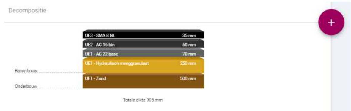
Figure 3: Example of an object decomposition in PIM with requirements at various levels
